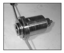
Pull seal sleeves (39) out of their fittings in the crankcase. Take seal case (38) out of seal sleeve (39).
