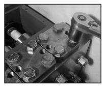
Loosen screws (58C), take plugs (58) out of valve casing with two screws.
