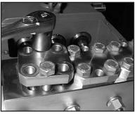
Take plugs (58) out of valve casing (50) by tightening screws (58C) against valve casing with two screws.
