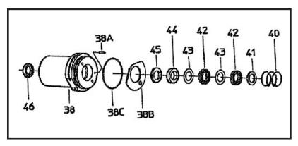
15) Remove grooved seal (46) from seal sleeve. Take pressure spring (40), support disc (41), seal unit (42, 43, 44) and pressure ring (45) out of seal sleeve (38). Remove leakage gasket (38B) from serated pin (38A) on seal sleeve (38). Replace worn parts from kit # 09224. **IMPORTANT!** The leakage gasket (38B) must be fitted to the seal sleeve (38) so that the bevelled surface of the gasket (38B) faces outward.
