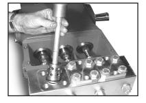
Take out valve assemblies (51 & 52) using either valve tool (part #07662) or a stud bolt (M16).
