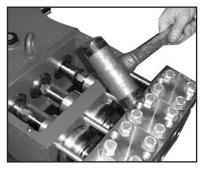
With a rubber mallet tap the back of the valve casing (50) and pull the valve casing off the stud bolt (49).
