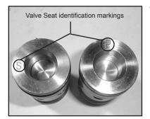
7) When reassembling: The inlet valve seat (51C) is 1mm smaller in diameter than the discharge valve seat (52C). Inlet valve seats are marked "S" and always have to be installed first. Discharge valve seats are marked "P" and are always to be installed on top of inlet valve. Plugs (58) are to be tensioned down evenly with screws (58C) in a crosswise pattern at 155 ft.-lbs. (210 Nm).
