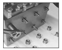
Loosen nuts (49A) with a 24mm socket wrench.
