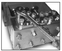
1) Loosen and remove screws (58C) with a 24mm socket wrench.
