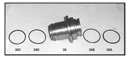
14) Remove and replace O-rings (39A, 39C) on support rings (39B, 39D).
