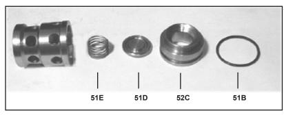
Check surfaces of valve plate (51D), valve seat (51C, 52C), O-rings (51B, 58A) and replace worn parts.
