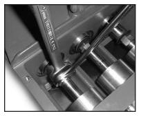
11) Using a 27mm wrench, separate the plunger (36) from the crosshead (25). NOTE: DO NOT loosen the three (3) plungers (36) before the the valve casing has been removed otherwise the plunger could hit against the spacer pipe (51F) when pump is being turned.
