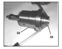
13) Use two screwdrivers to pry the seal case (39) from the seal sleeve (38).
