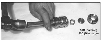
5) Valve seats (51C and 52C) are pressed out of spacer pipe (51F) by hitting the valve plate (51D) with a socket extention.
