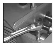
Remove cover plate (30) with a 10mm socket wrench.
