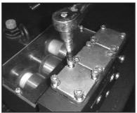
Unscrew inner hexagon screws (56A), remove plug (56) and pressure spring (54).
