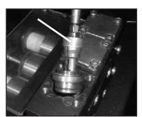
2) Using either a pin spanner or pliers, take out complete discharge valve (52), tension spring (53) and suction valve (51). The spring tension cap (51D/52D) is screwed together with valve seat (51A/52A). Remove spring tension cap, remove spring (51C/52C) and valve plate (51B/52B) The seal ring (51E/52E) is snapped onto the valve plate. Check sealing surfaces and o-rings (51F/52F/57). Replace worn parts.
