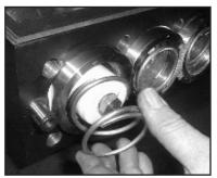
6) Take tension spring (42) out of seal sleeve (40).
