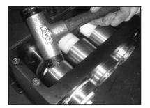
5) Remove seal sleeves (40) from the fittings in the crankcase, by tapping seal sleeve (40) out of the crancase with a rubber mallet.
