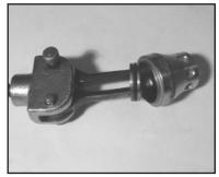
With a valve puller remove the valve seat (37) and o-ring (38) replace if worn. If excessive pitting is seen, replace the worn parts. Check valve seat o-ring (38) for wear and replace as necessary.
