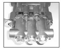
4. Drain the oil from the pump. Turn the pump over to remove the four manifold stud nuts (46) with a 19mm wrench.
