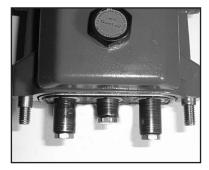
15. Before replacing pump manifold (29), first rotate crankshaft (18) until two outside plungers (24A) extend evenly forward. Next lubricate v-sleeves (50) in the rear v-sleeve housing (48) and slide housing over plungers. Lubricate ceramic plungers with a light film of oil. Carefully and evenly slide manifold over plungers and press manifold firmly against crankcase (1). Replace manifold stud bolts (45), washers (47) and nut (46) and tighten to 59 ft.-lbs. (80 Nm).
