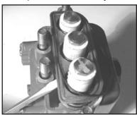
10. With a flat headed screwdriver remove the weep return plate (48). Remove the o-ring (49) and check for wear.
