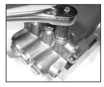
1. With a 22mm socket, remove the three discharge (43) and three inlet (41) manifold plugs.
