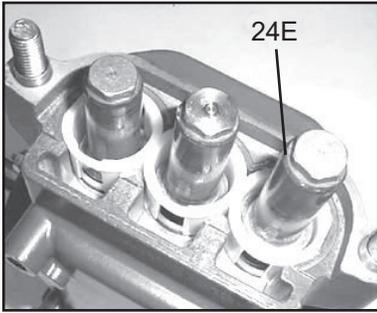
13. Replace copper ring (24E) onto plunger bolt (24B). Slide plunger bolt assembly (24) into ceramic plunger (24A). Apply a light film of loc-tite to plunger bolt threads and place plunger assembly onto stainless steel plunger base (22) and tighten to 247 in.-lbs. (28 Nm).
