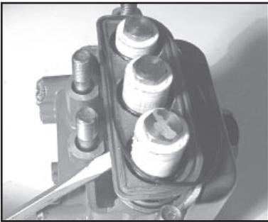
10. With a flat headed screwdriver remove the weep return plate (48). Remove the o-ring (49) and check for wear.
