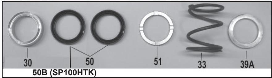
9. Remove the spacer (39A), pressure spring (33), support ring (51), sleeves (50/50B for SP100HTK only), and pressure ring (30), from the manifold (29) and check for wear.
