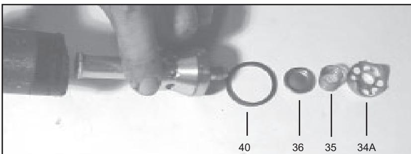
7. Remove the o-ring, (40), valve plate (36), valve spring (35), spring retainer (34A). Check valve retainer o-ring (40) for wear.
