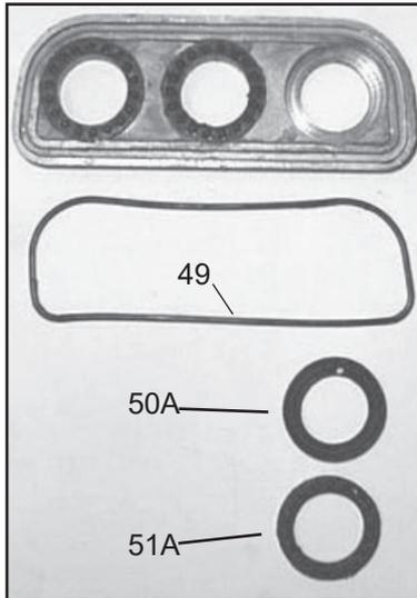
11. Inspect seals (50A), seal support ring (51A) and O-ring (49) and replace as necessary.
