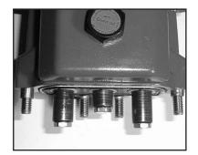
14. Before replacing pump manifold (29), first rotate crankshaft (18) until two outside plungers (24A) extend evenly forward. Next lubricate v-sleeves (50) in the rear v-sleeve housing (48) and slide housing over plungers. Lubricate ceramic plungers with a light film of oil. Carefully and evenly slide manifold over plungers and press manifold firmly against crankcase (1). Replace manifold stud bolts (45), washers (47) and nut (46) and tighten to 35 ft.-lbs. (47.5 Nm).
