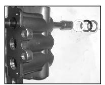
Turn the manifold (29) over. Using a 15mm socket, tap out the v-sleeves, Insert v-sleeve (31 & 31A), support rings (32), and pressure rings (30) through back of manifold.
