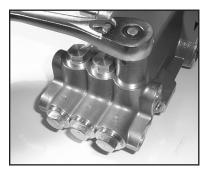
1. With a 22mm socket, remove the three discharge (43) and three inlet (41) manifold plugs. Check o-ring (44) for wear and replace as necessary.
