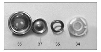
If pitted or worn, replace inlet valve seats (36), valve plates (37), springs (35) and spring retainers (34). Re-insert items 34-38 into valve adapter (39). Install valve assembly (34-40) into manifold (29). Reinstall manifold plugs (43) and torque plugs to 52 ft.-lbs. (70 Nm).
