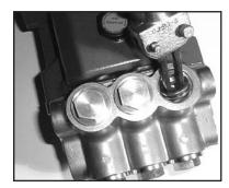
Use a small slide hammer to remove valve seats (37) from manifold (29). Inspect valve plates (36) and valve seats (37) for wear. If excessive pitting is seen, replace the worn parts. Check valve seat o-ring (38) for wear and replace as necessary. Tighten manifold plugs (41 and 43) to 52 ft.-lbs. (70 Nm).
