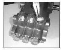
2. Remove the discharge spring retainer (34), valve spring (35), and valve plate (36).
