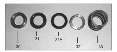
Inspect and clean the manifold and pressure ring. Reinstall the pressure ring (30) with the groved side pointed towards the front. Insert v-sleeves (31/31A), support ring (32), and pressure spring (33) into the manifold (29).
