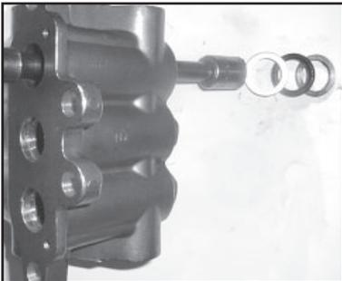
7. Turn the manifold (29) over. Using a 15mm socket, tap out the v-sleeves. Insert v-sleeve (31 & 31A), support rings (32), and pressure rings (30) through back of manifold.
