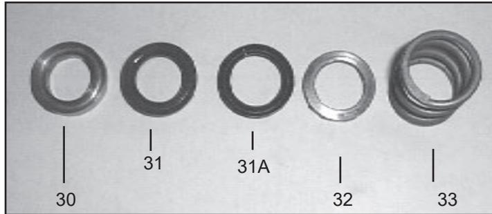
8. Inspect and clean the manifold and pressure ring. Reinstall the pressure ring (30) with the grooved side pointed towards the front. Insert v-sleeves (31/31A), support ring (32), and pressure spring (33) into the manifold (29).
