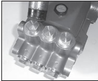
5. Tap the back of the manifold (29) with a rubber mallet to dislodge, and slide off the pump.
