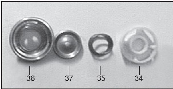
9. If pitted or worn, replace inlet valve seats (36), valve plates (37), springs (35) and spring retainers (34). Re-insert items 34-38 into valve adapter (39). Install valve assembly (34-40) into manifold (29). Reinstall manifold plugs (43) and torque plugs to 52 ft.-lbs. (70 Nm).
