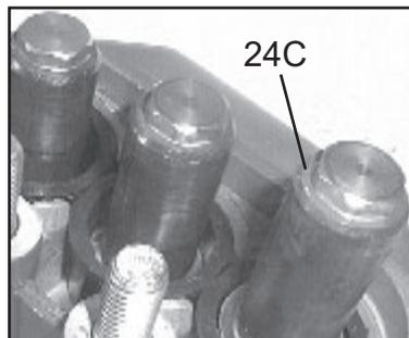
12. Replace copper ring (24C) onto plunger bolt (24B). Slide plunger bolt assembly into ceramic plunger (24A). Apply a light film of loc-tite to plunger bolt threads and place plunger assembly onto stainless steel plunger base (22) and tighten to 200 in.-lbs. (22.5 Nm).
