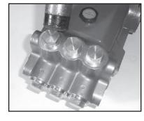
Tap the back of the manifold (29) with a rubber mallet to dislodge, and slide off the pump.
