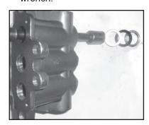
7. Turn the manifold (29) over. Using a 15mm socket, tap out the v-sleeves (31), support rings (32), and pressure rings (30) through back of manifold.
