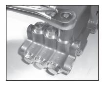
With a 22mm socket, remove the three discharge (43) and three inlet (41) manifold plugs. Check o-rings (42 and 44) for wear and replace as necessary.
