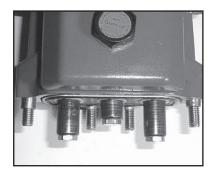
14. Before replacing pump manifold (29), first rotate crankshaft (18) until two outside plungers (24A) extend evenly forward. Next lubricate v-sleeves (50) in the rear v-sleeve housing (48) and slide housing over plungers. Lubricate ceramic plungers with a light film of oil. Carefully and evenly slide manifold over plungers and press manifold firmly against crankcase (1). Replace manifold stud bolts (45), washers (47) and nut (46) and tighten to 35 ft.-lbs. (47.5 Nm).
