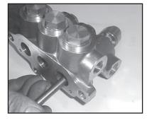
6. From the front inlet valve ports, remove the inlet valve assembly (34-40) and pressure springs (33).
