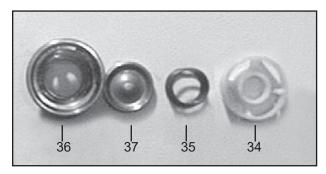
9. If pitted or worn, replace inlet valve seats (36), valve plates (37), springs (35) and spring retainers (34). Re-insert items 34-38 into valve adapter (39). Install valve assembly (34-40) into manifold (29). Reinstall manifold plugs (41) and torque plugs to 52 ft.-lbs. (70 Nm).
