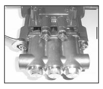
4. Drain the oil from the pump. Turn the pump over to remove the four manifold stud nuts (46) with a 17mm wrench.
