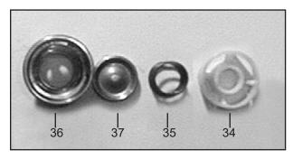
9. If pitted or worn, replace inlet valve seats (36), valve plates (37), springs (35) and spring retainers (34). Re-insert items 34-38 into valve adapter (39). Install valve assembly (34-40) into manifold (29). Reinstall manifold plugs (41) and torque plugs to 52 ft.-lbs. (70 Nm).
