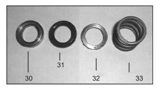
8. Inspect and clean the manifold (29) and pressure ring (32). Reinstall the pressure ring (30) with the groved side pointed towards the front. Insert v-sleeves (31), support ring (32), and pressure spring (33) into the manifold.
