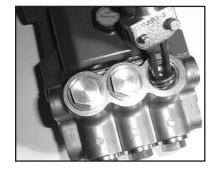
3. Using a small slide hammer remove valve seats (37) from manifold (29). Inspect valve plates (36) and valve seats (37) for wear. If excessive pitting is seen, replace the worn parts. Check valve seat o-ring (38) for wear and replace as necessary. Tighten manifold plugs (43) to 52 ft.-lbs. (70 Nm).
