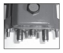
14. Before replacing pump manifold (29), first rotate crankshaft (18) until two outside plungers (24A) extend evenly forward. Next lubricate v-sleeves (50) in the rear v-sleeve housing (48) and slide housing over plungers. Lubricate ceramic plungers with a light film of oil. Carefully and evenly slide manifold over plungers and press manifold firmly against crankcase (1). Replace manifold stud bolts (45), washers (47) and nut (46) and tighten to 35 ft.-lbs. (47.5 Nm).
