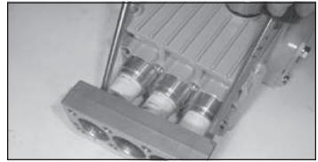
Using two screwdrivers, gently pry seal cases (21) out of the valve casing (26) or intermediate casing (25). Press grooved rings (23) and support rings (24) out of intermediate casing (25) using a screwdriver. Check O-rings (21A/25B). Examine seals (23). Replace worn seals.
