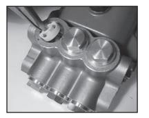
2. Remove the discharge spring retainer (34), valve spring (35), and valve plate (36).
