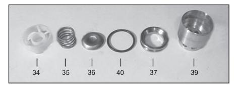
Inspect and clean the valve assembly parts. If pitted or worn, replace inlet valve seats (37), valve plates (36), spring (35) and spring retainers (34). Reinsert items 34-38 into valve adapter (39).
