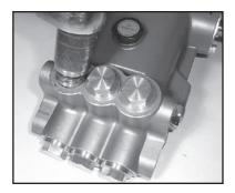
With a 22mm socket, remove the three discharge (43) and three inlet (41) manifold plugs. Check o-rings (42 & 44) for wear and replace as necessary.
