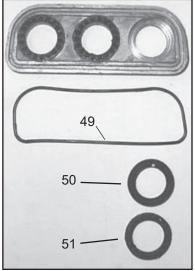
9. The rear V-sleeve housing (48) may be removed by prying evenly outward with a flat screwdriver. After slipping housing over plunger, inspect rear v-sleeves (50), support rings (51) and O-ring (49) and replace as necessary.
