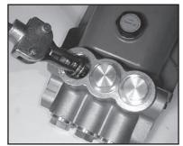
Use a small slide hammer to remove valve seats (37) from manifold (29). Inspect valve plates (36) and valve seats (37) for wear. If excessive pitting is seen, replace the worn parts. Check valve seat o-ring (38) for wear and replace as necessary.
