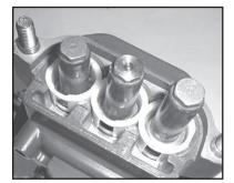
10.Inspect ceramic plunger (24A) tips for wear. If necessarv. replacement of the ceramic plungers may be accomplished by removing the plunger bolt assemblies (24B and 24C) with a 13mm wrench. Ceramic plungers should now slide off the stainless steel plunger base (22). Excessive resistance to plunger removal may be overcome by heating the stainless steel plunger base. This will melt any excess loc-tite beneath the ceramic plunger allowing easy removal.
