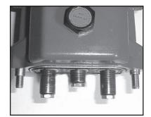
13.Before replacing pump manifold (29), first rotate crankshaft (18) until two outside plungers (24A) extend evenly forward. Next lubricate rear v-sleeves (50) and support ring (51) in the rear v-sleeve housing (48) and slide housing over plungers. Lubricate ceramic plungers with a light film of oil. Carefully and evenly slide manifold over plungers and press manifold firmly against crankcase (1). Replace manifold stud bolts (45), washers (47) and nut (46) and tighten to 35 ft.-lbs. (47.5 Nm).
