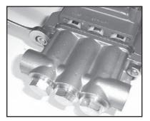
4. Drain the oil from the pump. Turn the pump over to remove the two manifold stud nuts (46) with a 17mm wrench.
