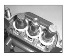
10.Inspect ceramic plunger (24A) tips for wear. If necessarv, replacement of the ceramic plungers may be accomplished by removing the plunger bolt assemblies (24B and 24C) with a 13mm wrench. Ceramic plungers should now slide off the stainless steel plunger base (22). Excessive resistance to plunger removal may be overcome by heating the stainless steel plunger base. This will melt any excess loc-tite beneath the ceramic plunger allowing easy removal.
