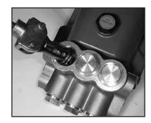
3. Use a small slide hammer to remove valve seats (37) from manifold (29). Inspect valve plates (36) and valve seats (37) for wear. If excessive pitting is seen, replace the worn parts. Check valve seat o-ring (38) for wear and replace as necessary.
