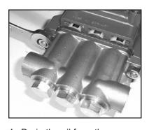
4. Drain the oil from the pump. Turn the pump over to remove the two manifold stud nuts (46) with a 17mm wrench.
