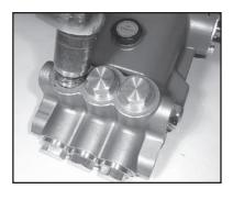
With a 22mm socket, remove the three discharge (43) and three inlet (41) manifold plugs. Check o-rings (42 & 44) for wear and replace as necessary.
