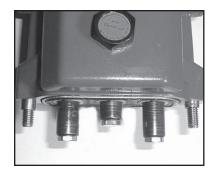
13. Before replacing pump manifold (29), first rotate crankshaft (18) until two outside plungers (24A) extend evenly forward. Next lubricate rear v-sleeves (50) and support ring (51) in the rear v-sleeve housing (48) and slide housing over plungers. Lubricate ceramic plungers with a light film of oil. Carefully and evenly slide manifold over plungers and press manifold firmly against crankcase (1). Replace manifold stud bolts (45), washers (47) and nut (46) and tighten to 35 ft.-lbs. (47.5 Nm).
