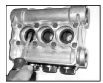
Remove the pressure rings (24) and v-sleeves (23) from the valve casing (26).
