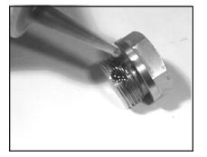
Remove the o-ring (31). Inspect all parts for wear and replace as necessary. Apply one drop of loctite 243 to the valve plugs (32) and tighten to 107 ft. lbs. (145 Nm).
