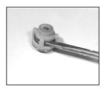
By inserting a small screwdriver between the valve seat (27) and the valve spring retainer (30), the valve assembly can be separated.
