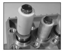
Check surfaces of plunger (16). Damaged surfaces cause accelerated seal wear. Deposits of all kinds must be removed from the plungers.
