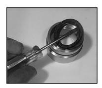
Remove the weep grooved seal (23) out of the seal adaptor (20). Check O-rings (21). **IMPORTANT!** The grooved seal (23) on the highpressure side is to be fitted carefully into the valve casing (26) using a screwdriver. Under no circumstances must the seal surface in the valve casing or the seal lip be damaged.
