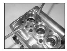
6) Remove seal adaptors (20) and weep return rings (25) from the valve casing.
