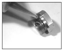
Remove the o-ring (31). Inspect all parts for wear and replace as necessary. Apply one drop of loctite 243 to the valve plugs (32) and tighten to 125 ft. lbs. (170 Nm).
