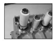
Check surfaces of plunger (16). Damaged surfaces cause accelerated seal wear.
