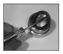
8) Remove the weep grooved seal (23) out of the seal adaptor (20). Check O-rings (21).
