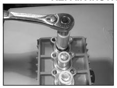
10) If the plunger pipe (16B) is worn, remove tension screw (16D) and remove along with plunger pipe (16B). Check and clean plunger surface (16A), check oil scraper (16H). Cover thread of tension screw (16D) with a thin film of Loctite and tighten carefully to 247 in.-lbs. (28 Nm).
