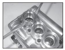
Remove seal adaptors (20) and weep return rings (25) from the valve casing.
