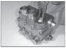
Using needle nose pliers, remove the inlet and discharge valve assemblies (27A). Note: It may become neccesary to remove the valve seat (27) from the valve casing using a slidehammer.
