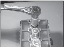
If the plunger pipe (16B) is worn, remove tension screw (16D) and remove along with plunger pipe (16B). Check and clean plunger surface (16A), check oil scraper (16H). Cover thread of tension screw (16D) with a thin film of Loctite and tighten carefully to 247 in.-lbs. (28 Nm).
