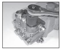
With a socket wrench, remove the three discharge valve plugs and three inlet valve plugs (32). Inspect the o-ring (33) for wear and replace if damaged.
