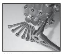
Use a 8mm allen wrench to remove the 8 socket head cap screws (34). Carefully slide the valve casing (26) out over the plungers.
