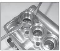
) Remove seal adapters (20) and weep return rings (25) from the valve casing.
