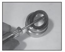
Remove the weep grooved seal (23B) together with pressure ring (24) out of the seal adapter (20). Check O-rings (21).
