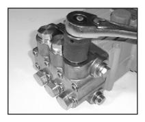
With a socket wrench, remove the three discharge valve plugs and three inlet valve plugs (32). Inspect the o-ring (33) for wear and replace if damaged.
