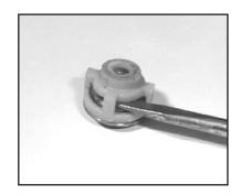
3) By inserting a small screw driver between the valve seat (27) and the valve spring retainer (30), the valve assembly can be separated.
