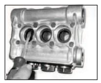
7) Remove the pressure rings (24) and v-sleeves (23 - Note: P422 & P423 pumps have a spacer ring) from the valve casing (26).
