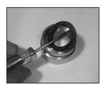
Remove the weep grooved seal (23 or 23B) together with pressure ring (24) P420 and P425 only) out of the seal case (20). Check O-rings (21). **IMPORTANT!** The grooved seal (23) on the highpressure side is to be fitted carefully into the valve casing (26) using a screwdriver. Under no circumstances must the seal surface in the valve casing or the seal lip be damaged.
