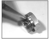
4) Remove the o-ring (31). Inspect all parts for wear and replace as necessary. Apply one drop of loctite 243 to the valve plugs (32) and tighten to 107 ft.-lbs. (145 NM).
