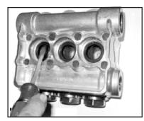
Remove the pressure rings (24) and v-sleeves (23 - Note: P422 & P423 pumps have a spacer ring) from the valve casing (26).
