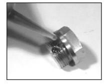
Remove the o-ring (31). Inspect all parts for wear and replace as necessary. Apply one drop of loctite 243 to the valve plugs (32) and tighten to 125 ft. lbs.
