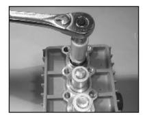
10) If the plunger pipe (16B), or oil seal (19) is worn, remove tension screw (16D) and remove along with plunger pipe (16B). Check and clean plunger surface (16A), check oil scraper (16H). Remove the gear seal adapter (20A) and, if necessary, replace oil seals with seal lips facing crankcase (1).Cover thread of tension screw (16D) with a thin film of Loctite and tighten carefully to 26 ft.-lbs. (35NM).
