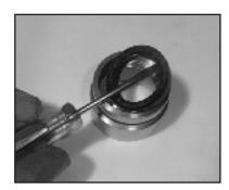
Remove the weep grooved seal (23 or 23B) together with pressure ring (24 \_ P420 and P425 only) out of the seal adaptor (20). Check O-rings (21). **IMPORTANT!** The grooved seal (23) or respectively grooved seal pack (23A) on the high-pressure side is to be fitted carefully into the valve casing (26) using a screwdriver. Under no circumstances must the seal surface in the valve casing or the seal lip be damaged.
