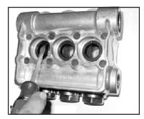
Remove the pressure rings (24) and v-sleeves (23 -Note: P422 & P423 pumps have a support ring) from the valve casing (26).
