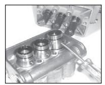
8. Remove weep return rings (#25) from the plungers (#16). Remove the seal case (#20) from either crankcases (#1) or manifold (#26) by using a screwdriver as shown above. NOTE: If there are deposits of any kind (i.e., lime deposits) in the valve casing, be certain the weep holes in the weep return ring (#25) and valve casing (#26) have not been plugged.
