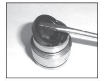
12. Use a flat screw driver to pry the oil seals (#19) loose from the seal case (#20).
