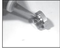
5. Apply one drop of Loctite 243 to valve plugs (32) and tighten to 55 ft.-lbs. (75 Nm). For pumps manufactured prior to 5/97 tighten plugs to 37 ft-lbs. (50 Nm).
