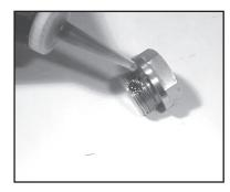
5. Apply one drop of Loctite 243 to valve plugs (#32) and tighten to 55 ft.-lbs. (75 Nm).
