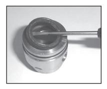
Remove the weep grooved seals (#23A for P314, P321 & P327 and #23 for P318, P324, P330 & P334) from the seal case (#20).
