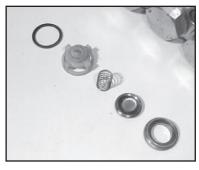
Remove each o-ring (#31). Inspect all parts for wear and replace as necessary. Reassemble valve assy's (#32X) & place in valve casing (#26).
