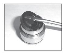
12. For P314, P321 & P327 pumps, use a flat screw driver to pry the oil seals (#19) loose from the seal case (#20).
