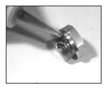
Apply one drop of Loctite 243 to the valve plugs (32) and tighten to 55 ft.-lbs. (75 Nm).
