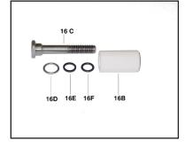
8. Check surfaces of plunger pipe (16B). A damaged surface will cause accelerated wear on the seals. Deposits of any kind must be carefully removed from the plunger surface. A damaged plunger must be replaced!
