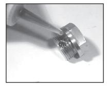
Apply one drop of Loctite 243 to the valve plugs (32) and tighten to 55 ft.-lbs. (75 Nm).
