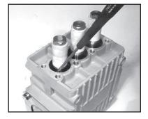
If the crankcase oil seals (19) are to be replaced, they can be removed by prying loose with a flat screwdriver. Take care not to make contact with the plunger.
