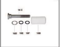
Check surfaces of plunger pipe (16B). A damaged surface will cause accelerated wear on the seals. Deposits of any kind must be carefully removed from the plunger surface. A damaged plunger must be replaced!
