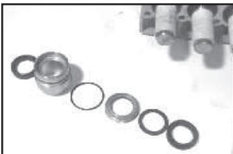
7. Remove the weep return ring (25), pressure ring (24), and v-sleeve (23) from the valve casing (26). Remove the rear v-sleeve (23A) from the seal case (20). Inspect pressure ring (24) behind the seal case (20). Inspect all parts, including o-ring (21) for wear and replace as necessary.
