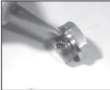
4. Remove the o-ring (31) Inspect all parts for wear. Apply one drop of Loctite 243 to the valve plugs (32) and tighten to 55 ft.-lbs. (75 NM).
