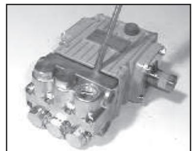
6. Carefully slide the valve casing (26) out over the plungers.
