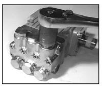
With a 22mm socket wrench, remove the (3) discharge valve plugs and (3) inlet valve plugs (32) Inspect the o-ring (33) for wear and replace if damaged.
