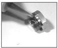
Remove the o-ring (31). Inspect all parts for wear and replace as necessary. Apply one drop of Loctite 243 to the valve plugs (32) and tighten to 55 ft.-lbs. (79 Nm).
