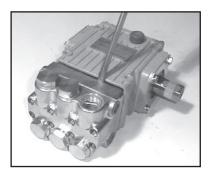
Carefully slide the valve casing (26) out over the plungers.
