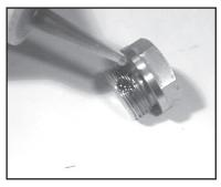
4. Remove the o-ring (31). Inspect all parts for wear and replace as necessary. Apply one drop of Loctite 243 to the valve plugs (32) and tighten to 55 ft.-lbs. (79 Nm).
