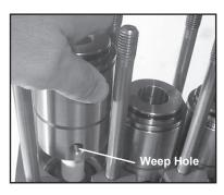
12) Replace complete seal sleeve (35)/seal case (37) assembly into crankcase (1). Make sure that the weep hole points downward. Note:
