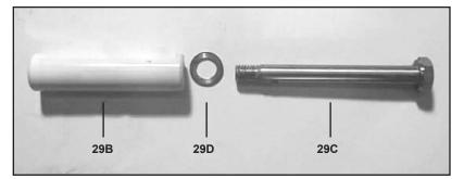
12) Check plunger surface (29B). If plunger pipe is worn out, loosen tension screws (29C) with a 15mm socket and pull off plunger pipe to the front. Clean front surface of plunger (29B) thoroughly. Apply a small drop of locktite to tension screw. Put a **new** crush washer (29D) onto tension screw. Put a thin coat of glue (Loctite) on the ring (or ceramic plunger side) and tighten screw to 26 ft.-lbs. (35 NM).
