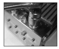
5) Tighten up tension plugs (48) to 107 ft.-lbs. (145 NM).
