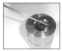
10) Remove leakage seal (36) from the seal sleeve. If worn or damaged replace with new seal.
