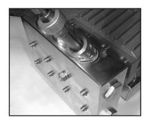
Take out discharge valve assemblies (46) by pulling them upwards out of the valve casing (43) with a snap-ring tongs or any other pull-off device. Then remove inlet valves in the same way.
