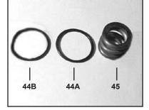
2) Remove the support ring (44B), O-ring (44A) and tension spring (45).
