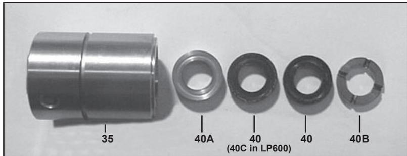
11) Remove the guide ring (40A), v-sleeves (40/40C), and support ring (40B), from the seal sleeve. Examine seals carefully and replace if worn. Clean surfaces of seal sleeves (35) which come in contact with the crankcase (1) and sealing surfaces of valve casing (43).
