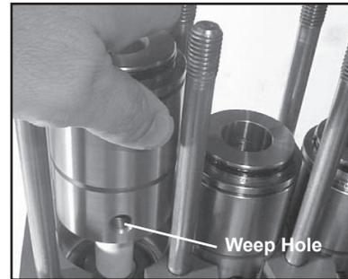
12) Check plunger surface (29B). If plunger pipe is worn out, loosen tension screws (29C) with a 15mm socket and pull off plunger pipe to the front. Clean front surface of plunger (29B) thoroughly. Apply a small drop of locktite to tension screw. Put a **new** crush washer (29D) onto tension screw. Put a thin coat of glue (Loctite) on the ring (or ceramic plunger side) and tighten screw to 26 ft.-lbs. (35 NM).
