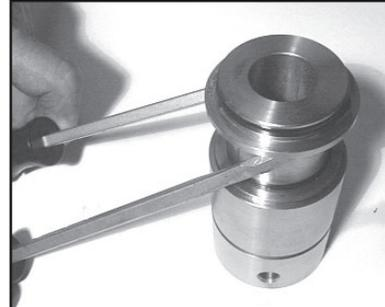
8) Remove seal case (37) from seal sleeve (35).
