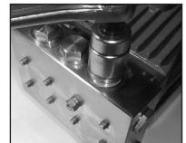
5) Tighten up tension plugs (48) to 107 ft.-lbs. (145 NM)
