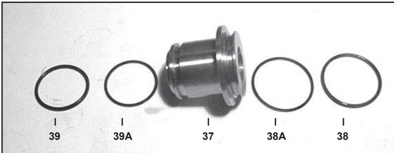
9) Check O-rings (39 & 38) and support rings (39A & 38A) on seal case (37).
