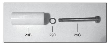
Check plunger surface (29B). If plunger pipe is worn, loosen tension screws (29C) and pull off plunger pipe to the front. Clean front surface of plunger (25) thoroughly. Apply a thin coat of Loctite to the tension screw threads (29C). Note: Care must be taken that no glue gets between the plunger pipe (29B) and the centering sleeve (29A). Add new copper ring (29D).
