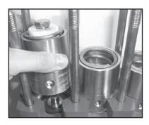
Place new plunger pipe (29B) carefully through the oiled seals and push seal sleeve (35) with plunger pipe into the crankcase guide. Note: Make sure weep hole is facing down.
