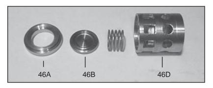
4. Loosen valve seats (46A) from spacer pipe (46D) by lightly hitting the valve plate (46B) with a plastic stick. Check sealing surface and replace worn parts. Reassemble with new O-rings (44A) and oil them before installing. Tighten up tension plugs (48) to 107 ft.-lbs. (145 NM).
