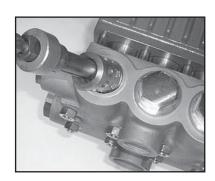
3. Remove the complete valve assembly (46A-46D) with valve pullers.
