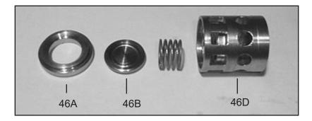
4. Loosen valve seats (46A) from spacer pipe (46D) by lightly hitting the valve plate (46B) with a plastic stick. Check sealing surface and replace worn parts. Reassemble with new O-rings (44A) and oil them before installing. Tighten up tension plugs (48) to 107 ft.-lbs. (145 NM).
