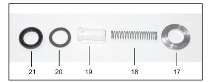
Remove the guided p-valve, (19), valve springs (18), v-sleeves (21) and pressure rings (20). Inspect for wear and replace as necessary. Remove the spacer ring (17) from the plungers (8).
