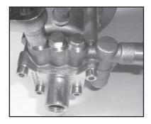
1. With a 14mm socket wrench, remove the three discharge valve plugs (22).Inspect the valve plug o-rings (23) for wear, and replace as necessary.
