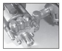
3. With a crescent wrench, remove the injector retainer (47). Inspect the o-ring (46) for wear and replace as necessary.
