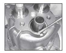
8. If the crankcase oil seals (15) are to be replaced, they can be removed by prying loose with a screwdriver. Take care not to make contact with the plunger (8) and pry out the oil seals from their housing.
