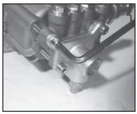
8. Next, remove the four manifold bolts (40) with a 6mm allen wrench.
