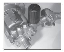
3. With a crescent wrench, remove the kickback valve spring retainer (47). Inspect the o-ring (46) for wear and replace as necessary. Remove the kickback valve spring (43), kickback valve cone (42), and the o-ring (41) from the manifold (35). Inspect the parts for wear and replace as necessary.
