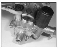
With a 14mm socket wrench, remove the three discharge valve plugs (22). Inspect the valve plug o-rings (23) for wear, and replace as necessary.
