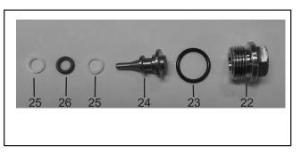
7. Remove the piston (24), o-ring (26), and backup rings (25). Remove the bypass valve seat (28). Inspect the parts for wear and replace as necessary. IMPORTANT! Make sure that the shoulder on bypass valve seat (28) is facing the discharge plug (22).
