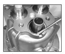
12. If the crankcase oil seals (15) are to be replaced, they can be removed by prying loose with a screwdriver. Take care not to make contact with the plunger (8) and pry out the oil seals from their housing. Seals should not be reinstalled until after step #13.
