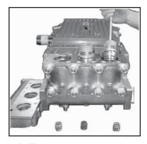
Take out pressure springs (57A). Pull out assembled valves (51 & 52) with valve puller.
