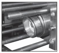
8) Take out the seal case (38) from the valve casing (50) and check o-rings (38A) (if necessary secure two screwdrivers in the front o-ring groove to extract seal casing from valve casing). Coat seals with silicon grease before installing.
