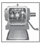
11) Take out plungers and seal sleeves as described above. Drain the oil by taking off the plug (12). After removing the clip ring (33B), lever out the seal retainer (33) and radial shaft seal (32) with a screwdriver. Open hose adapter (K11) and remove gear cover (K3) by removing the socket head cap screws (K5). Remove the cooling vane plate (K1) by removing the screws (K4)
