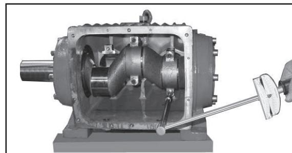
14) Reassemble in reverse order. Thread the long end of the crankshaft together with the inner bearing rings into the crankcase; then mount outer bearing ring (20) and spacer ring (22A). Mount connecting rod halves in their exact original position and tighten at 37 Ft-lbs. (50 Nm).
