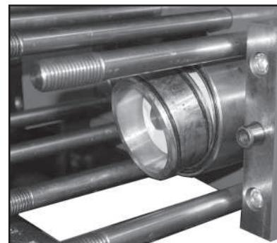
8) Take out the seal case (38) from the valve (if necessary secure 2 screwdrivers in the front O-ring groove to extract seal casing from valve casing). Coat seals with silicon grease before installing.
