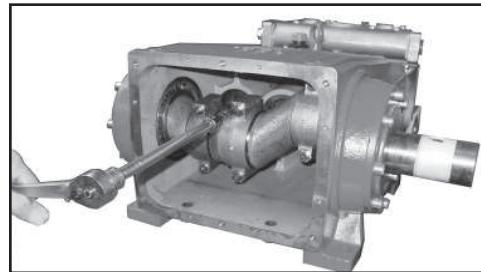
11) Take out plungers and seal sleeves as described above. Drain the oil by taking off the plug (12). After removing the clip ring (33B), pry out the seal retainer (33) with a screwdriver. Open hose adaptor (K11) and remove gear cover (K3) and the cooling vane plate (K1) by removing the screws (K4).
