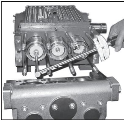
9) Lightly coat the seal sleeve with anti-corrosive grease (e.g. molykote no. Cu-7439) in its fitted area towards the crankcase. Insert the seal sleeves in to their crankcase fittings. Lightly coat the threads of the tension screw (36C) with thread glue and insert it together with a new copper ring (36D) through the ceramic pipe. Turn the pump by hand until the plunger (25) rests against the plunger pipe. Tighten the tension screw at 30 Ft-lbs. (40 Nm).
