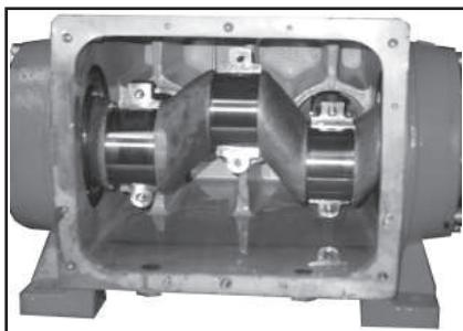
13) Push connecting rod halves together with the crosshead as far as possible into the crosshead guide. Take out bearing cover (14/14A) and push out crankshaft taking particular care that the con rod doesn't get bent. Check surfaces on the connecting rods (24), crankshaft (22) and crossheads (25). Check the surfaces of the crosshead guides in the crankcase for any unevenness.
