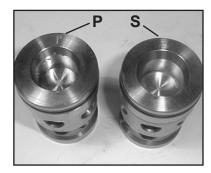
5. When reassembling: The suction valve seat (51C) is 1mm smaller in diameter than the discharge valve seat (52C). Suction valve seats are marked "S" and always have to be installed first. Discharge valve seats are marked "P" and are always tobe installed on top of suction valve. Plugs (58) are to be tensioned down evenly with screws (58C) in a crosswise pattern at 155 ft-lbs. (210 Nm).
