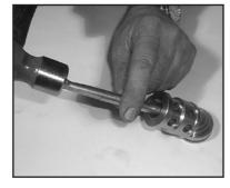
Valve seats (51C and 52C) are pressed out of spacer pipe (51F) by hitting the valve plate (51D/52D) with a bolt.
