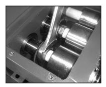
8. Separate plunger (36A) from crosshead (25) by means of one open-end wrench (M36).
