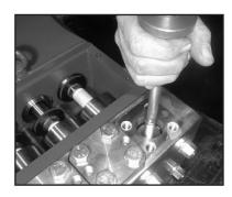
Take out tension spring (57) and complete valve (51) using either valve tool (part #07662) or stud bolt M16.
