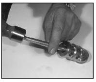
Valve seats (51C and 52C) are pressed out of spacer pipe (51F) by hitting the valve plate (51D) with a bolt.
