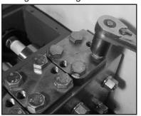
Loosen screws (58C), press plugs (58) out of valve casing with two screws - using them like "jack screws".
