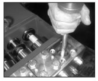
Remove tension spring (57) and complete valve assemblies (51 and 52) using either tool (part #07662) or stud bolt.
