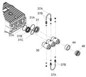
Take the seal tension spring (41) out of seal sleeve (36). Using a pliers, remove the clip ring (32) situated on the other side of the sleeve; then take out support ring (33) and grooved ring (35) using an extractor tool (either ø14 or ø16).
