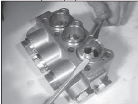
5. Using two screwdrivers, remove seal case (21)
