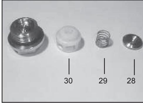
2. Remove the exposed spring tension cap (30) from valve seat by pushing it sideways with a screwdriver. Remove spring tension cap (30), valve spring (29), and valve plate (28).
