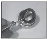
Remove the weep grooved seal (23B) together with pressure ring (24) out of the seal adaptor (20). Check O-rings (21). Coat new seals and o-rings with silicone grease.
