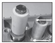
9) Check surfaces of plunger (16). Damaged surfaces cause accelerated seal wear. Deposits of all kinds must be removed from the plungers. **IMPORTANT!** Plunger surfaces are not to be damaged. If there are lime deposits in the pump, care must be taken that the drip-return bore in parts (25) and (26) ensure trouble-free drip-return.
