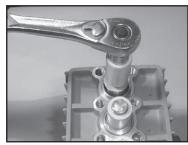
10) If the plunger pipe (16B), is damaged or worn, remove tension screw (16D) and plunger pipe (16B). Check and clean plunger surface (16A) and check flinger (16H). Cover thread of tension screw (16D) with a thin film of Loctite and tighten carefully to 22 ft.-lbs. (28 Nm).
