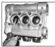
Remove the pressure rings (24) and grooved seals (23) from the valve casing (26).
