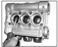
7) Remove the pressure rings (24) and grooved seals (23) from the valve casing (26).
