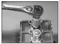
10) If the plunger pipe (16B), is damaged or worn, remove tension screw (16D) and plunger pipe (16B). Check and clean plunger surface (16A) and check flinger (16H). Cover thread of tension screw (16D) with a thin film of Loctite and tighten carefully to 22 ft.-lbs. (28 Nm).
