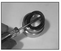
8) Remove the weep grooved seal (23B) together with pressure ring (24) out of the seal adaptor (20). Check O-rings (21). Coat new seals and o-rings with silicone grease.
