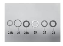
7. Remove the weep return ring (25), pressure ring (24), and v-sleeve (23) from the valve casing (26). Remove the rear v-sleeve (23A) and drip shield (23B) from the seal case (20). Inspect all parts, including o-ring (21) for wear and replace as necessary.
