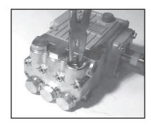
Using a needle nose pliers, remove the inlet and discharge valve assemblies (27-30). Inspect all parts for wear and replace as necessary.
